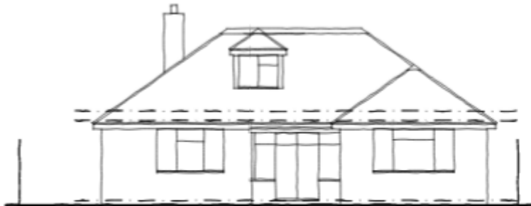
Existing Rear Elevation 1:100
